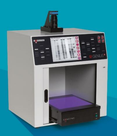
The **InGenius 3** gel documentation and analysis system is compact and easy to use. The system has a small footprint darkroom featuring a CCD camera, manual zoom lens and a filter drawer.
