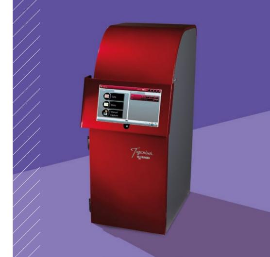
U:Genius 3 and U:Genius 3 EZ are compact imaging systems for gel documentation. U:Genius 3 provides an intelligent image capture and storage system.
